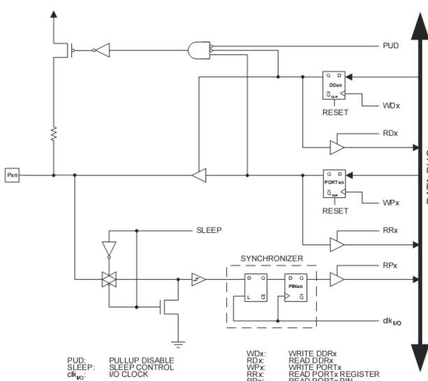
Note: 1. WPx, WDX, RRx, RPx, and RDx are common to all pins within the same port. clk<sub>I/O</sub>, SLEEP, and PUD are common to all ports.
